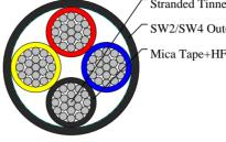
Stranded Tinned Copper Conductor
